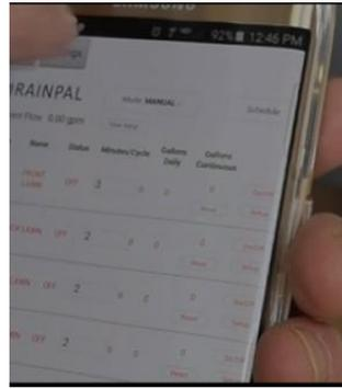
***Shown here, The Rainpal controller with its smart device Application user interface. The device can be accessed for monitoring, control, or configuration over the internet, on the local network, or as a direct hot spot access point within 100 feet from the controller. The Rainpal device comes in three models. The Rainpal Pro residential unit, the Rainpal Commercial unit, and the Rainpal Agricultural unit.***
